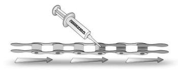
Apply the lube evenly on the mid part of the link. During first chain turns it will be distributed all over the whole surface. The consistency of the lube enables it to penetrate under the chain seals and thus reach all working areas of chain and sprockets. Do not apply excessive quantities of lube on particular links.
